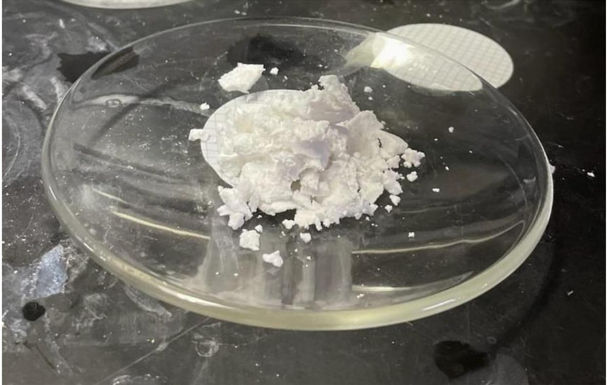
Figure 1 – Photograph of Lithium Carbonate Product from TLC Test Work
